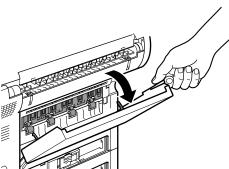
**2** Hold up the face-up tray slightly ① to release the lock pin ② ③ which is located on the right side of the tray.
