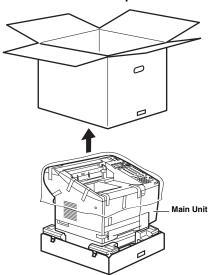
**5** Lift the main unit by gripping the handles on its right and left sides. (See "Moving the Machine", on p. 1-1.)
