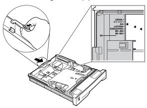
Before you load a stack of paper into the paper cassette, tap the leading edge of the paper stack on a flat surface so that the edges are evenly aligned.
