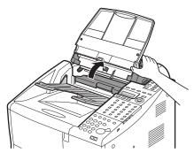
While holding the ADF cover open with one hand, use one finger of your other hand to gently push in the black, plastic loop to separate it from the stub on the machine.
