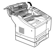
9 Use a soft, dry cloth to wipe clean the scanning glass, the white strip above, the rollers, and the area around the scanning glass.
