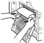
☐ After the paper's edge has rolled out, pull the paper forward carefully.
