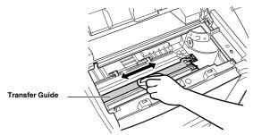
While holding the green label, flip the transfer guide up to its full extent. Wipe the edge of the transfer guide with a soft, clean cloth, to remove toner and paper dust from both sides of the transfer guide.
