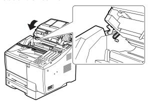
11 Place the end of the black, plastic loop over the end of the stub, so that it stays in place.
