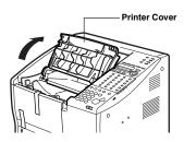
4 Remove the shipping tape of the MP tray and the printer cover.
