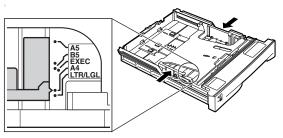
□ Push the stopper in the center of the paper size rear guide, and slide it to the mark indicating the desired paper size.
