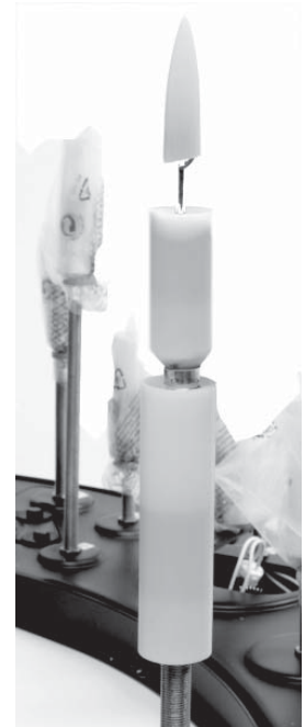
Flicker Bulb (installed)
