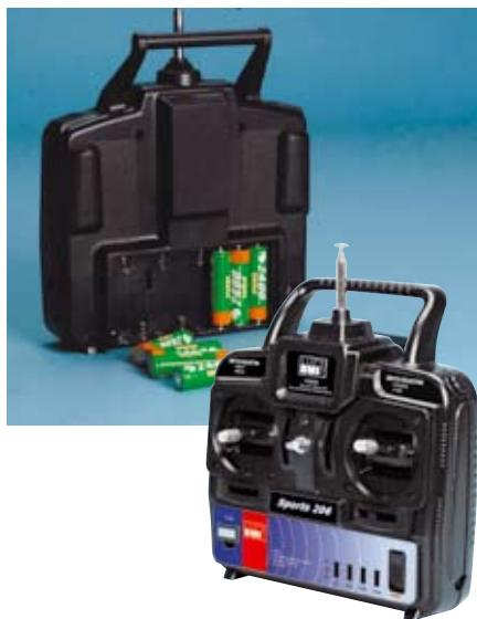
Prepare 8 PCS of AA Batteries and install them into the transmitter; pull out the antenna of the transmitter, and pull the throttle stick and its trim to Minimum position, and then turn on the power of the transmitter.
