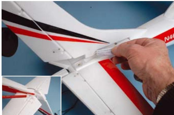
Take out the fin, and tear off the gummed paper. Insert and fit the fin into the appointed holes in the fuselage and the tail plane and fix this with glue. It is very important that the fin is mounted at 90° on the stabiliser.
