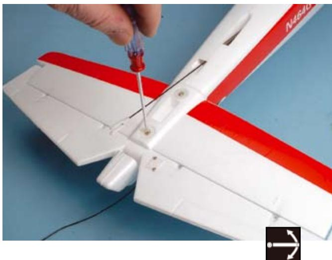
Take out the tail stabiliser, insert the tail flap into the fuselage and fit it with two screws slightly, the longer one in front the shorter one in back. It is important that the stabiliser has the same angle as the main wing.
