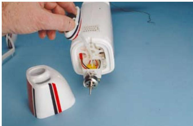
Take out the front landing gear and take off the head cover; fit the front landing gear to the motor board and buckle the clevis to the arm of the front landing gear.
