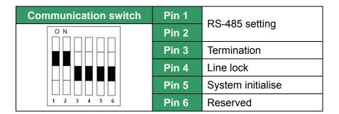
RS-485 is the interface that allows the PTZ camera to communicate with its control unit; the RS-485 configuration on the PTZ camera and the control unit must therefore
