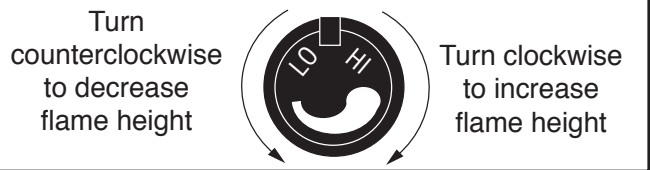
Fig. 16 Flame adjustment knob for Honeywell Valve.
