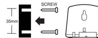
**IMPORTANT** — Before drilling the wall, check that there are no pipes or cables buried in the wall, that will be damaged by the drill. Do not drill directly above or below other electrical fittings unless you are sure that the cables to these are routed away from the drill position.
