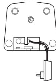
6. Plug the mains power adaptor into a (230V) mains socket and switch it on.
