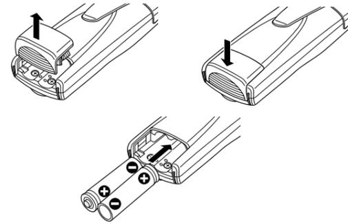
**IMPORTANT** — The batteries supplied with this product are rechargeable Ni-MH, 1300mAh. When replacing batteries, never use other types of batteries or conventional alkaline batteries.
