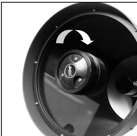
Figure 8-1 Rotate the collimation screw cover to access the three collimation screw.
