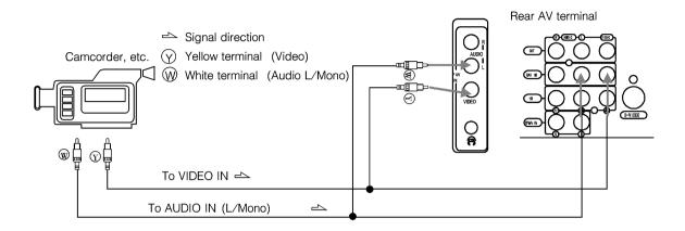
Connect AUDIO OUT (IN) of external equipment to LEFT/MONO IN (OUT) of your projection TV if that equipment doesn't have STEREO OUT (IN).
