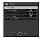
With Blue Screen on, the projection TV will display a blue background and mute automatically when no signal received. With Blue Screen off, the projection TV will display noise dots on the screen in the TV mode or the screen becomes dark in the AV mode when no signal is present.
