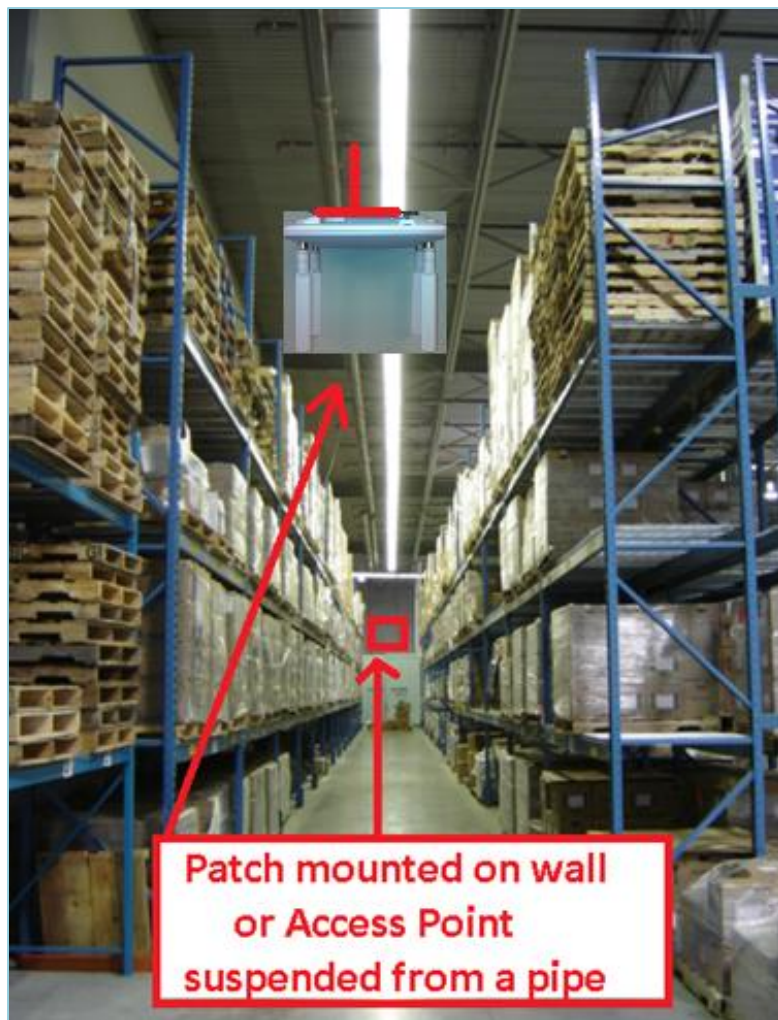
Figure 29: AP Placement in Warehouse
