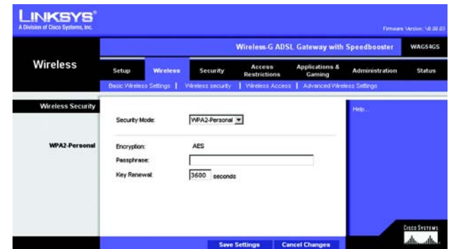
Figure 6-17: Wireless Security - WPA2-Personal
