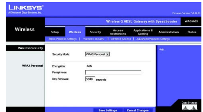
Figure 6-17 : Wireless Security - WPA2-Personal (Sécurité sans fil - WPA2-Personal)
