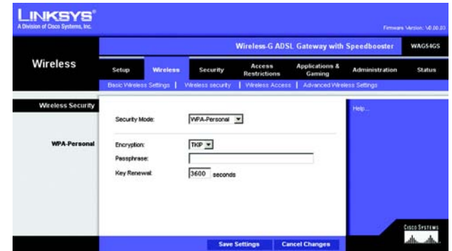
Figure 6-16: Wireless Security - WPA-Personal
