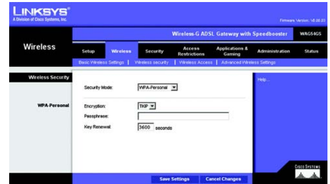
Figure 6-16 : Wireless Security - WPA-Personal (Sécurité sans fil - WPA-Personal)
