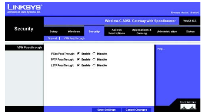
Figure 6-25 : VPN Passthrough (Intercommunication VPN)
