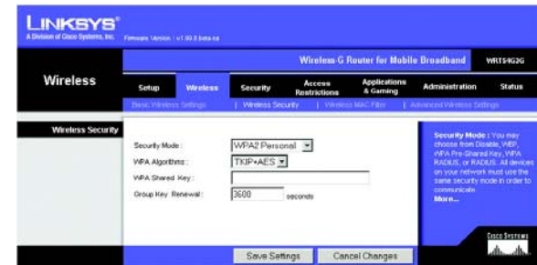
Figure 8-19: Wireless Tab - Wireless Security (WPA2 Personal)
