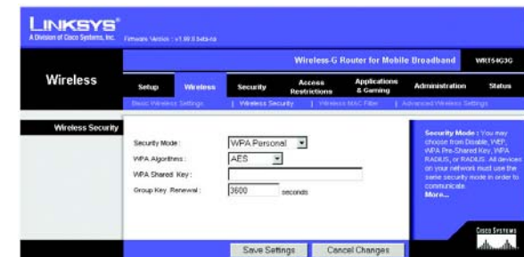
Figure 8-21: Wireless Tab - Wireless Security (WPA Personal - AES)
