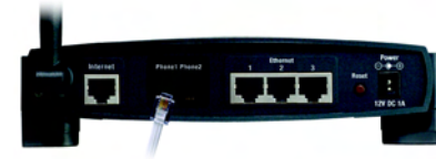
Figure 4-2: Connect a Telephone
