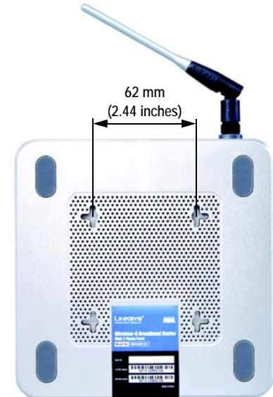
Figure 4-6: Measurement between Wall-Mount Slots
