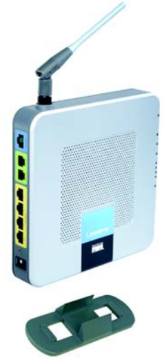
Figure 4-5: Attach the Stand to the Router
