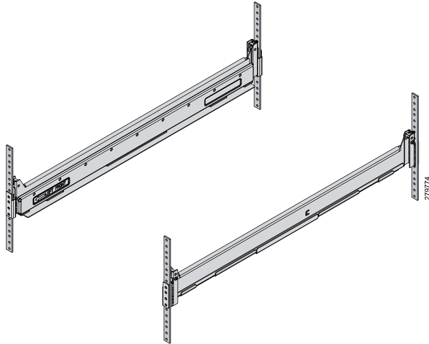
Figure 9: Round Hole Adapter and Rails Installed in a Rack
