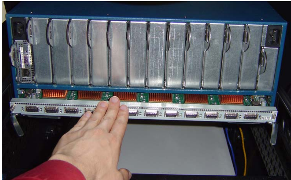
Figure 2-7: Inserting a Switch Card
