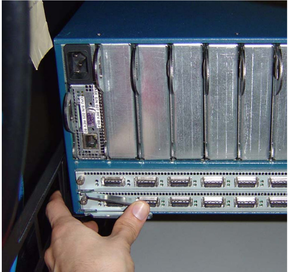
Figure 2-8: Closing Switch Ejector Levers
