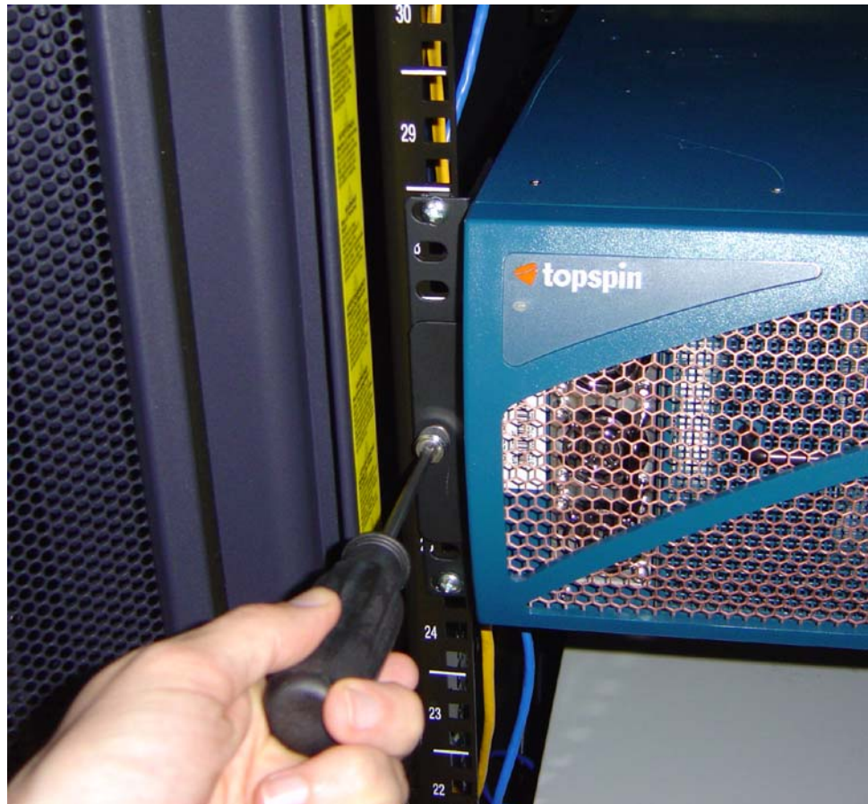
Figure 3-8: Securing the Chassis to the Rails
