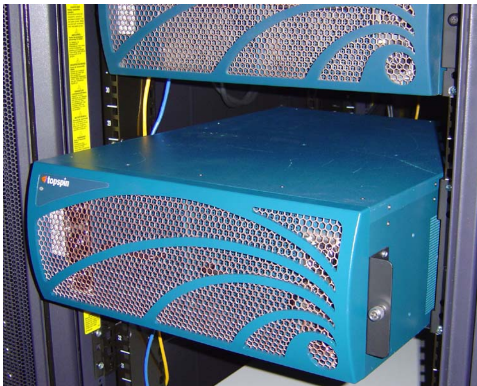
Figure 3-7: Sliding the Chassis onto the Rails
