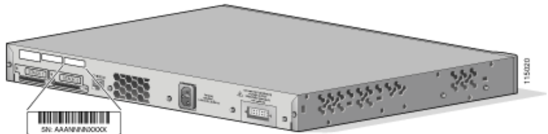
Figure 3-1 Catalyst 3750G-12S and 3750-12S-SD Switch Serial Number Location
