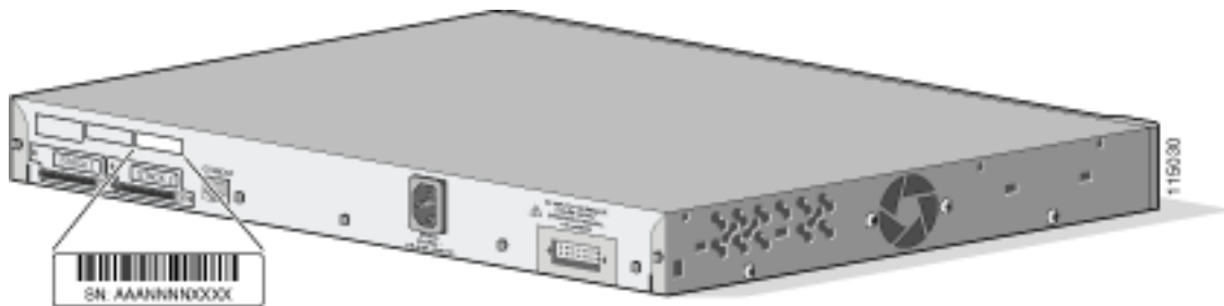
Figure 3-9 Catalyst 3750-48PS Switch Serial Number Location
