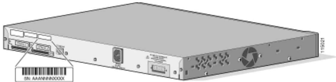
Figure 3-7 Catalyst 3750-24PS Switch Serial Number Location
