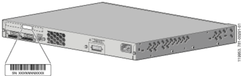
Figure 3-4 Catalyst 3750G-24PS and 3750G-24TS-1U Switches Serial Number Location
