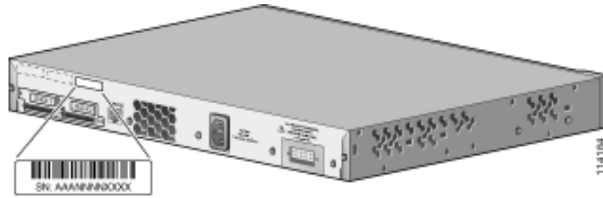
Figure 3-11 Catalyst 3750-48TS Switch Serial Number Location
