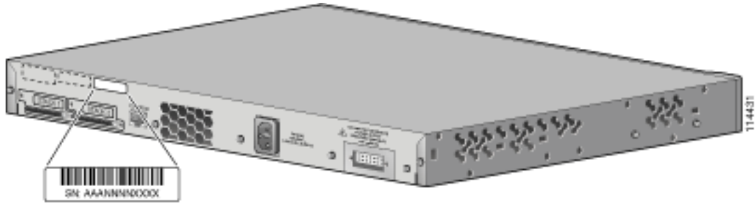
Figure 3-2 Catalyst 3750G-16TD Switch Serial Number Location
