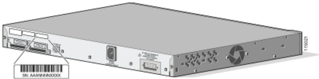
Figure 3-3 Catalyst 3750-24PS Switch Serial Number Location
