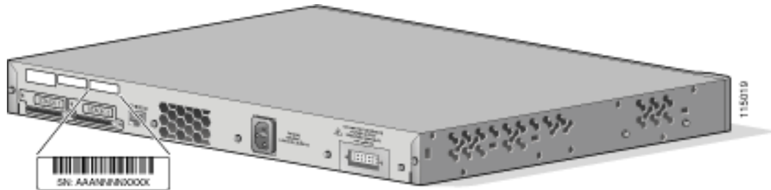
Figure 3-6 Catalyst 3750-24TS Switch Serial Number Location
