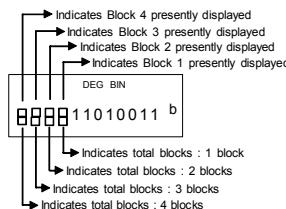
The block function comprises upper and lower block indicators. The upper indicator means current block position, and the lower indicator means total blocks for a result.
