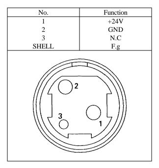
Connector used : TCS7960-53-2010 (Hoshiden) or equivalent Applicable connectors : TCP8927-63-1100 (Hoshiden) or equivalent
