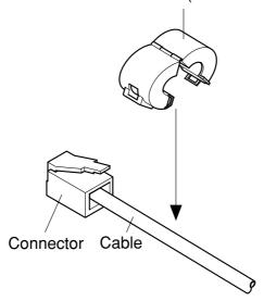
Pass the fastener through the ferrite core.
