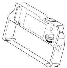
Holding the ribbon cassette so that the ribbon is facing down, install the cassette into the slip printer as shown in the illustration.
