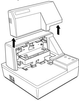
To replace the cover, slide it back down into position. Gently press down on the cover until you hear it click securely into place.
