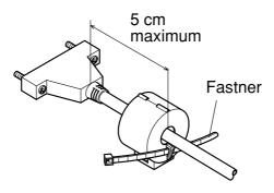
Loop the fastener around the cable and lock it. Use scissors to cut off any excess.
