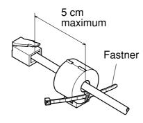
Loop the fastener around the cable and lock it. Use scissors to cut off any excess.
