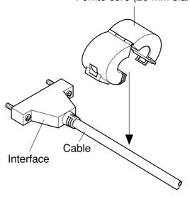
Pass the fastener through the ferrite core.
