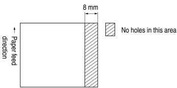
Do not use paper with perforations within the shaded area. Perforations may cause the paper sensor to erroneously report an out of paper condition.
