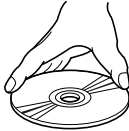
Proper way to hold the compact disc
