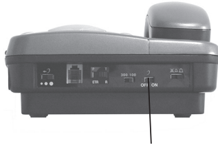
DIAGRAM #13 - Volume override switch
