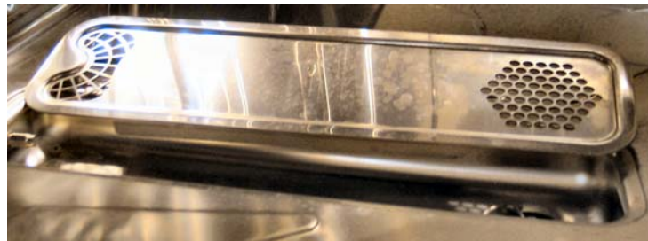
Drain Cover and Drain
