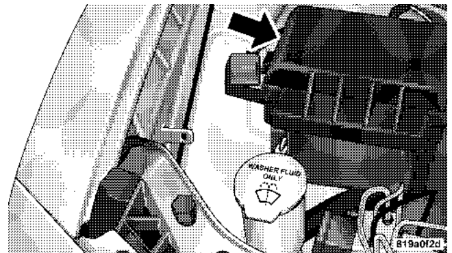
Front Power Distribution Center
