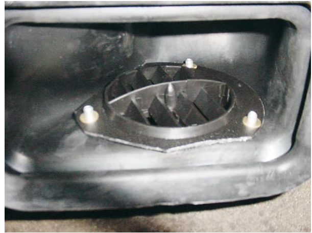
Figure 15a - V4 RND black installed in the duct transition
