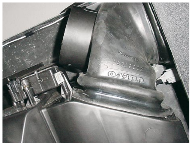
Figure 16 - Duct transition reinstalled
