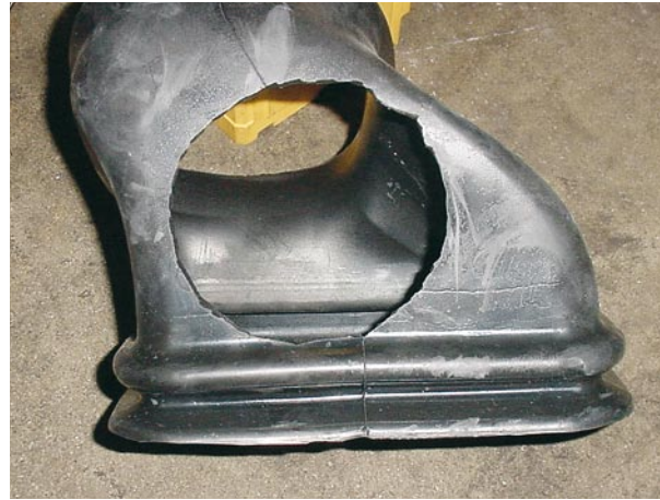
Figure 12 - Hole cut in duct transition
