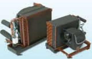
**AT-MU air handlers** are designed for use in fresh air make-up systems where outside air is drawn in by the air handler, cooled, dehumidified, and reheated to room temperature, then ducted to various areas.
