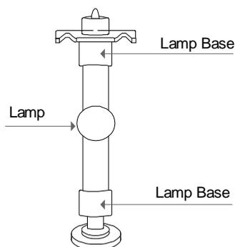
**⚠ Warning: Never touch the glass or white powder of the lamp as finger oil, dust or water will damage the lamp.**
