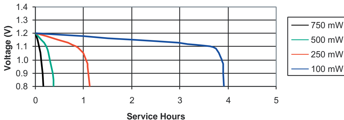
Discharge Characteristics at Various Power Drains
