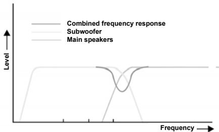
With the phase settings you can adjust the timing relationship between the subwoofer and main speakers. If either subwoofer or main speaker are slightly delayed in response in relation to the other, it can result in decreased bass output in the frequency response area where they overlap each other.
