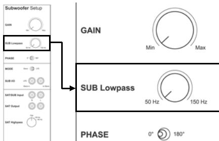
The **SUB Lowpass** control allows the frequency range of the subwoofer to be defined. Above the selected frequency the sound level decreases rapidly. The correct setting of this cut-off frequency is important for a well balanced combination of subwoofer and speakers.
