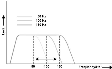
Matching the frequency responses of subwoofer and speakers has an important impact on the overall sound quality, when integrating a subwoofer into a audio-video-system. In general a large, floor-standing speaker still has significant output in the deeper bass range, whereas a very small speaker will not be able to reproduce deep bass at all. In the first case a bump in the overlapping area will cause a louder or even bloated sound while in the second case an acoustic hole will be experienced.
