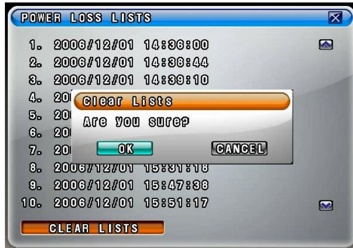
Fig.6-19 POWER LOSS LISTS Message
