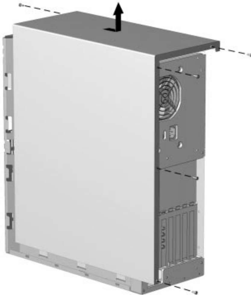
Figure 6-5. Removing the J Hood
