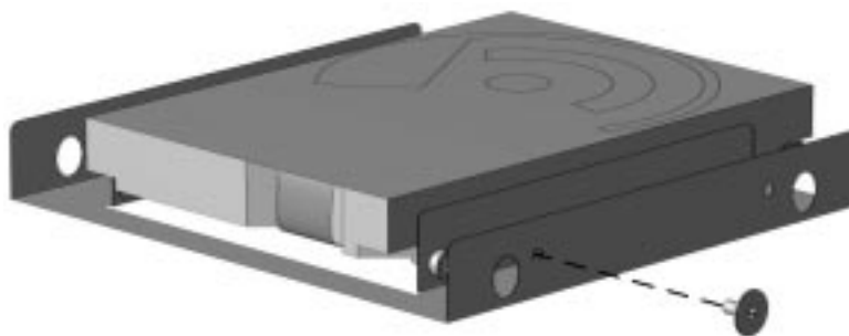
Figure 6-40. Installing the Wafer Screw on the Right Side of the Bracket
