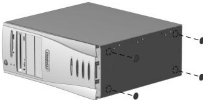
Figure 6-2. Installing the Feet
