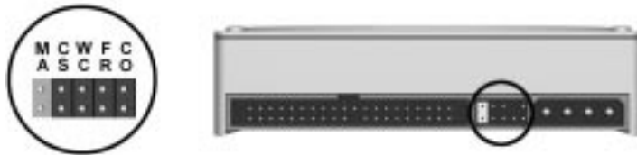
Figure 7-16. 3.2-GB Maxtor EIDE Hard Drive Jumper Settings
