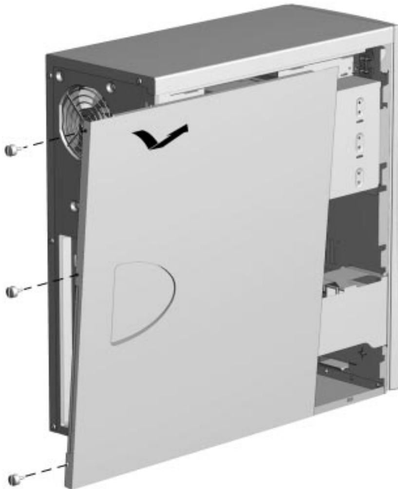
Figure 6-4. Removing the Access Panel
