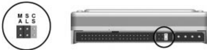
Figure 7-12. 2.1-GB Western Digital EIDE hard drive Jumper settings
