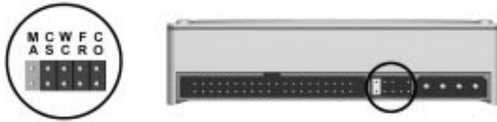
Figure 7-21. 3.2-GB Maxtor Ultra ATA Hard Drive Jumper Settings
