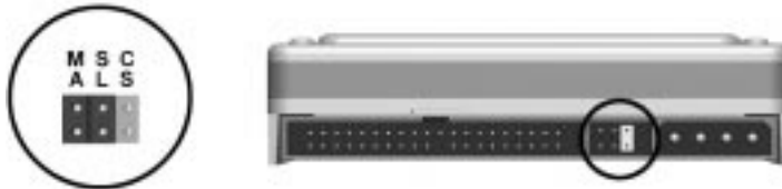
Figure 7-15. 3.2-GB Western Digital EIDE Hard Drive Jumper settings
