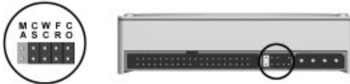
Figure 7-19. 2.1-GB Maxtor Ultra ATA Hard Drive Jumper Settings
