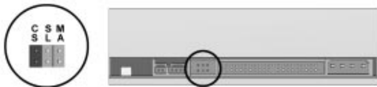
Figure 7-22. Jumper Pins for the 16X max EIDE CD-ROM Drives
