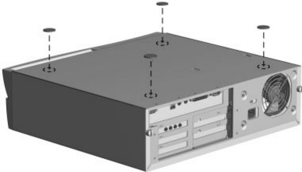
Figure 5-2. Installing the Feet
