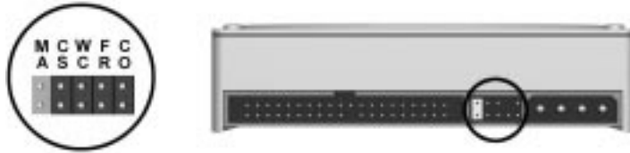
Figure 7-13. 2.1-GB Maxtor EIDE Hard Drive Jumper Settings
