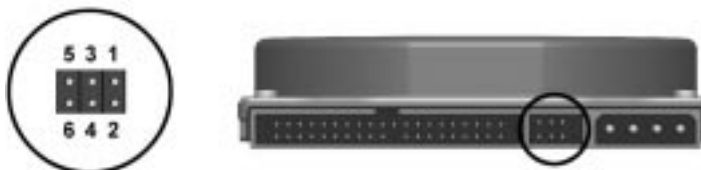
Figure 7-20. 2.4-GB Ultra ATA Hard Drive Jumper Settings
