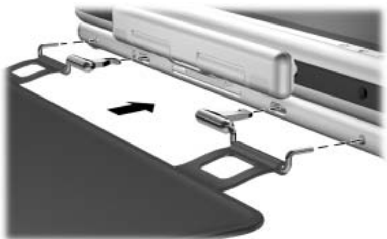
Attaching the screen protector to the keyboard
