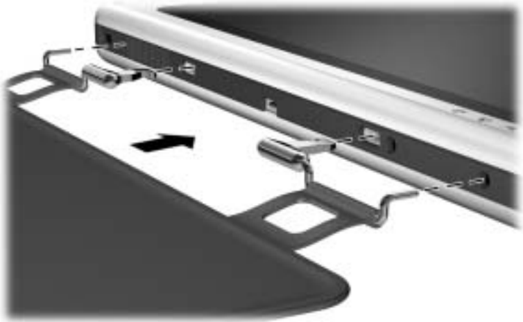
Attaching the screen protector to the tablet PC
