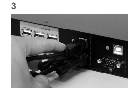
Connect KVM cable from computer system to KVM ports
