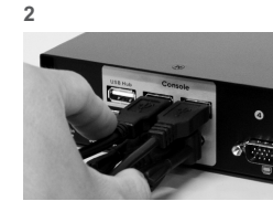
Connect console 1. Monitor 2. Mouse 3. Keyboard
