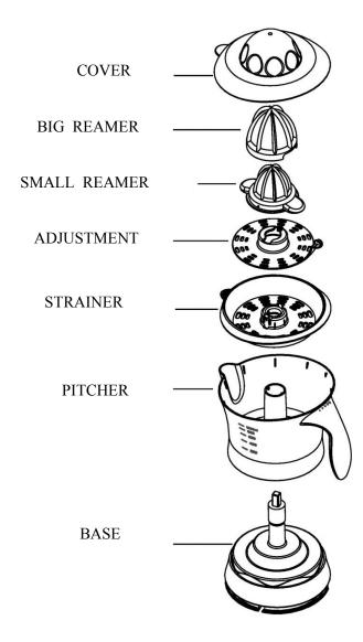
The two reamers are designed for squeezed various size citrus. A large size citrus need to press against the large reamer, if a small size citrus is squeezed, the large reamer is needed to remove and use the small reamer only.
