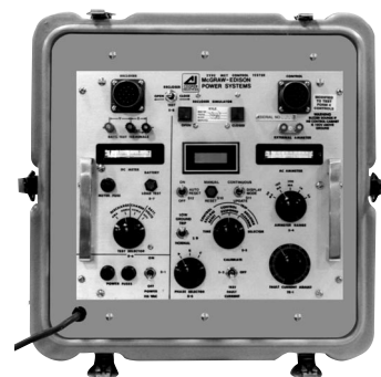
Figure 41. Kyle Type MET electronic recloser control tester.
