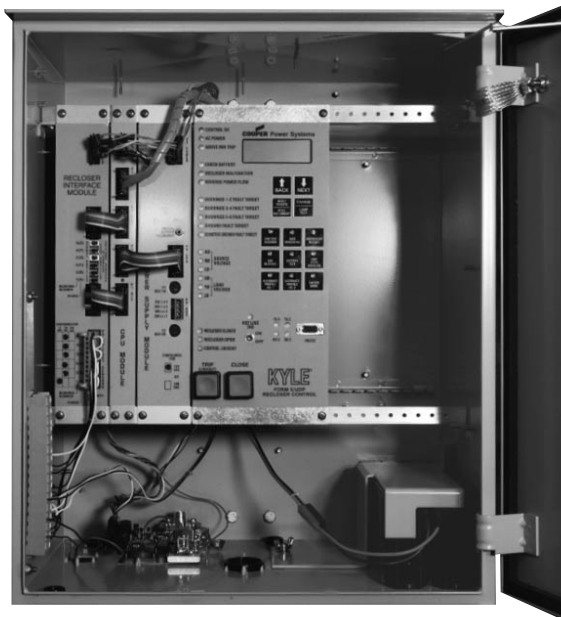
Figure 1. Kyle® Form 5/UDP microprocessor-based recloser control.
