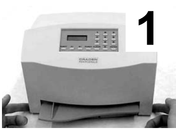
Push in on cabinet latches Rotate cabinet up and back.
