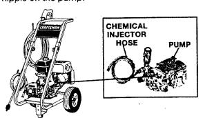
Connect high pressure hose to the quick connect outlet on pressure washer.
