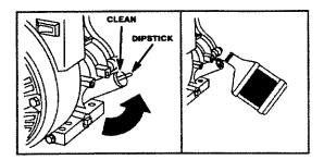
NOTE: When adding oil to the engine crankcase, use a high quality detergent oil classified "For Service SF, SG, SH rated SAE 30 weight. Use no special additives. Select the oil's viscosity grade according to your expected operating temperatures.
