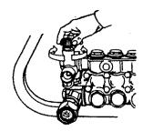
After using the pressure washer, it is recommended the pump, chemical injector and chemical line be flushed with clear water. To do so, simply place chemical injector hose in water and siphon for 1 to minutes.
