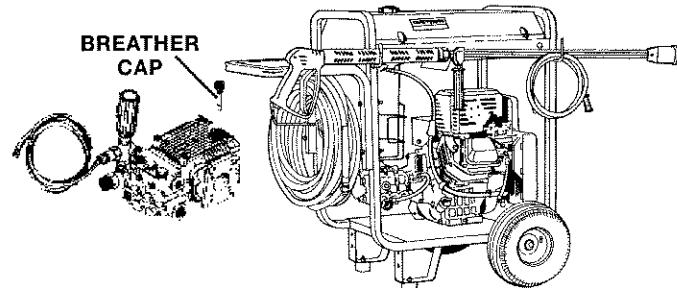
**▲ CAUTION:** Failure to replace the plug will result in serious pump damage.
