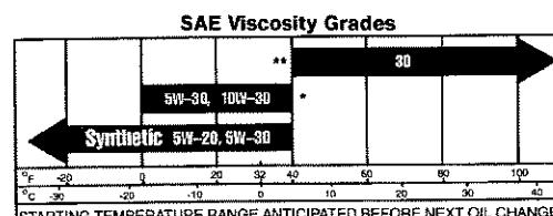
Air cooled engines run hotter than automotive engines. The use of multi-viscosity oil such as (10W-30, etc.) in ambient temperatures above 40°F (4°C) will result in higher than normal oil consumption. If multi-viscosity oil is used, check the oil level more frequently to prevent any possible engine damage due to lack of lubrication.
