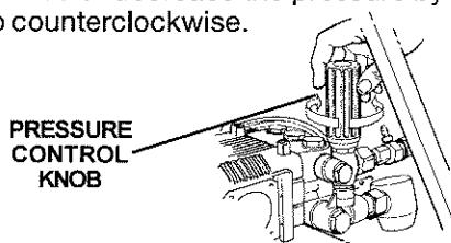
**NOTE:** The maximum pressure for the unit is factory adjusted. Do not attempt to adjust beyond this factory setting.
