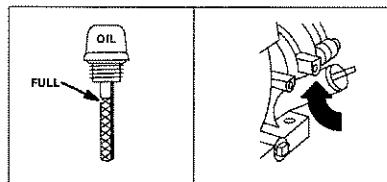
Do not clean engine with a forceful spray of water because water could contaminate fuel system. With a brush or cloth clean finger guard after every use to prevent engine damage caused by overheating.
