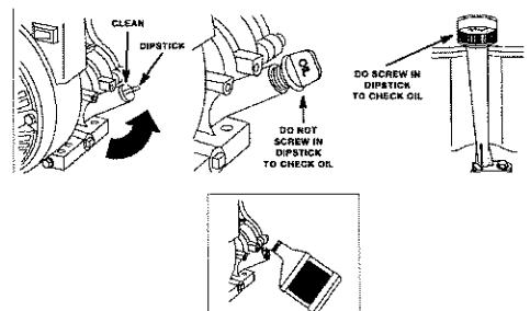
**NOTE:** When adding oil to the engine crankcase, use a high quality detergent oil classified 'For Service SF, SG, SH rated SAE 30 weight. Use no special additives. Select the oil's viscosity grade according to your expected operating temperatures.
