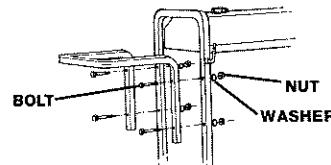
2. • Attach chemical basket to the pressure washer frame opposite side of muffler. Holes are provided on frame.
