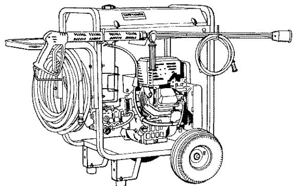
**NOTE:** Your unit's pump is shipped with a temporary plug that must be replaced with a breather cap. This plug is located over the pump's oil port. Unscrew and remove this plug. Remove the breather cap from the bag attached to the plug and install it in the pump's oil port.
