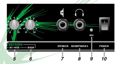
**7: SPEAKER:** Use this jack to connect the amplifier to an external speaker. The internal speaker is disconnected when this jack is used. The impedance of the external speaker must be 4 ohms or greater.
