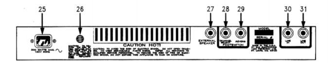
25: POWER CORD: Firmly plug the supplied, heavy-duty grounded power cord into this receptacle. When in use, be sure this cord is properly plugged into a safely-wired, grounded 120 volt, 60 cycle AC power outlet. DO NOT attempt to defeat the ground connection on this cable!
