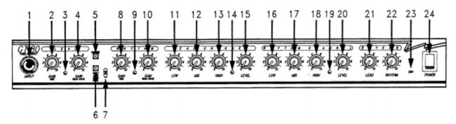
1: INPUT: Connect your guitar here using a shielded instrument cable.
