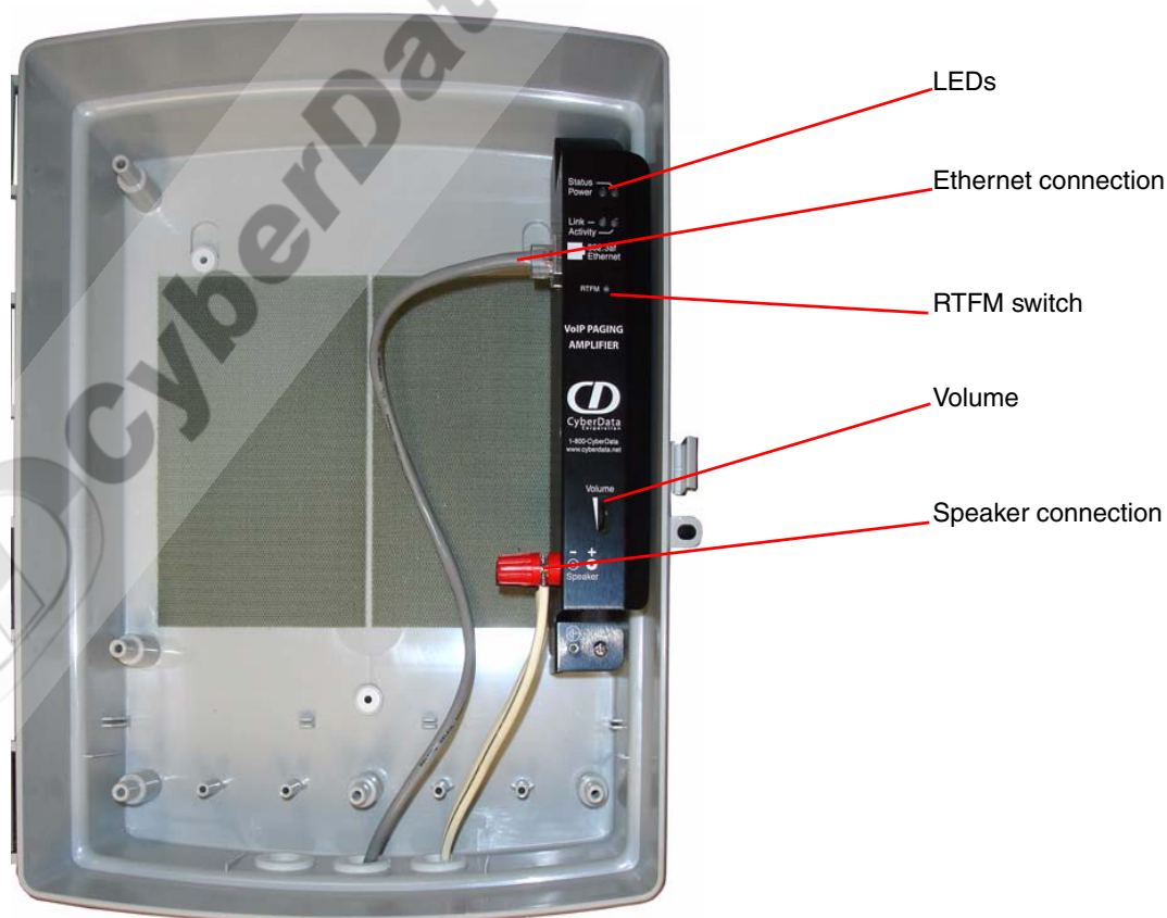
Figure 2-1. Loudspeaker Amplifier Components—PoE
