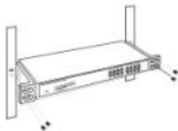
Figure 2. Mount the Switch in the rack.
