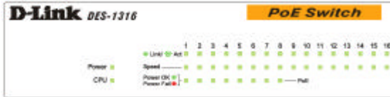
Figure 5. LED indicators of the Switch
