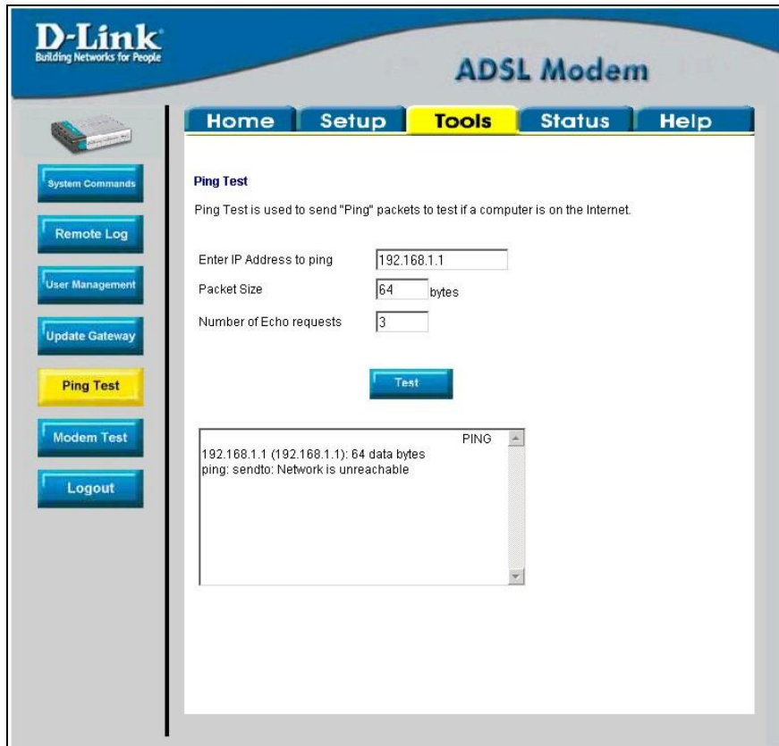
Figure 4-8. Tools – Ping Test window
