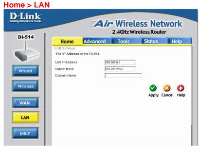
LAN is short for Local Area Network. This is considered your internal network. These are the IP settings of the LAN interface for the DI-514. These settings may be referred to as Private settings. You may change the LAN IP address if needed. The LAN IP address is private to your internal network and cannot be seen on the Internet.
