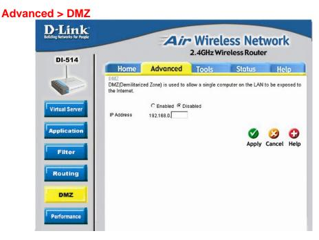
If you have a client PC that cannot run Internet applications properly from behind the DI-514, then you can set the client up to unrestricted Internet access. It allows a computer to be exposed to the Internet. This feature is useful for gaming purposes. Enter the IP address of the internal computer that will be the DMZ host. Adding a client to the DMZ (Demilitarized Zone) may expose your local network to a variety of security risks, so only use this option as a last resort.
