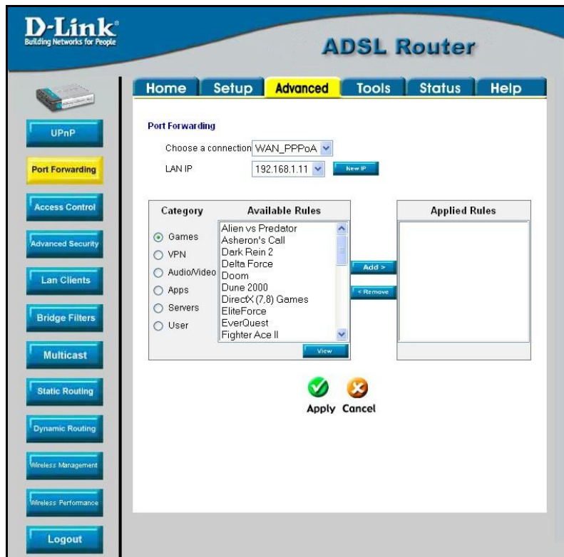
Figure 4-4. Advanced – Port Forwarding window
