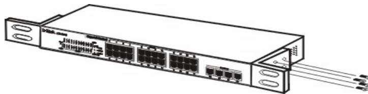
Figure 5. Use the screws provided, then use the equipment rack to mount the Switch in the rack.
