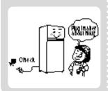
• After running the refrigerator for 2 ~ 3 Hours put food in the refrigerator.
