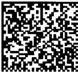
Bar Code W1c: DataMatrix
