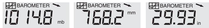
Displaying Units: Barometric Pressure Units: millibars (mb), millimeters (mm) and inches (in)
