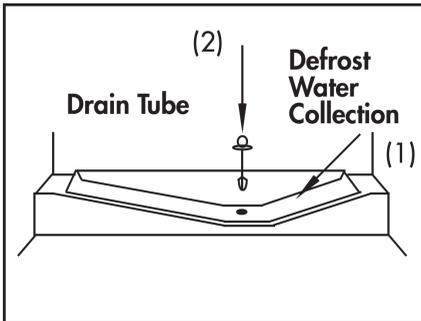
During defrosting water droplets may form at the back of the fridge compartment where the concealed evaporator is located. Some droplets may remain on the liner and refreeze when defrosting is completed.
