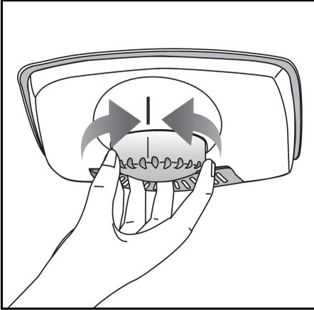
Operating temperatures are controlled by the thermostat knob (see diagram) located on the ceiling of the fridge compartment. Settings may be made from 1 to 5, 5 being the coldest position.
