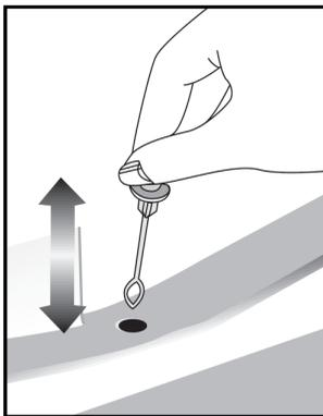
If at any time the defrost water does not drain from the collection channel, check to ensure that no food particles have blocked the drain tube.
