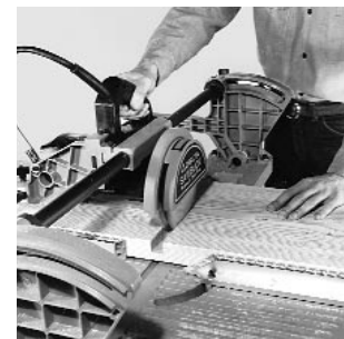
Special 31.62° miter stop and 33.85° bevel setting facilitates compound cutting standard 52°/38° crown moulding.
