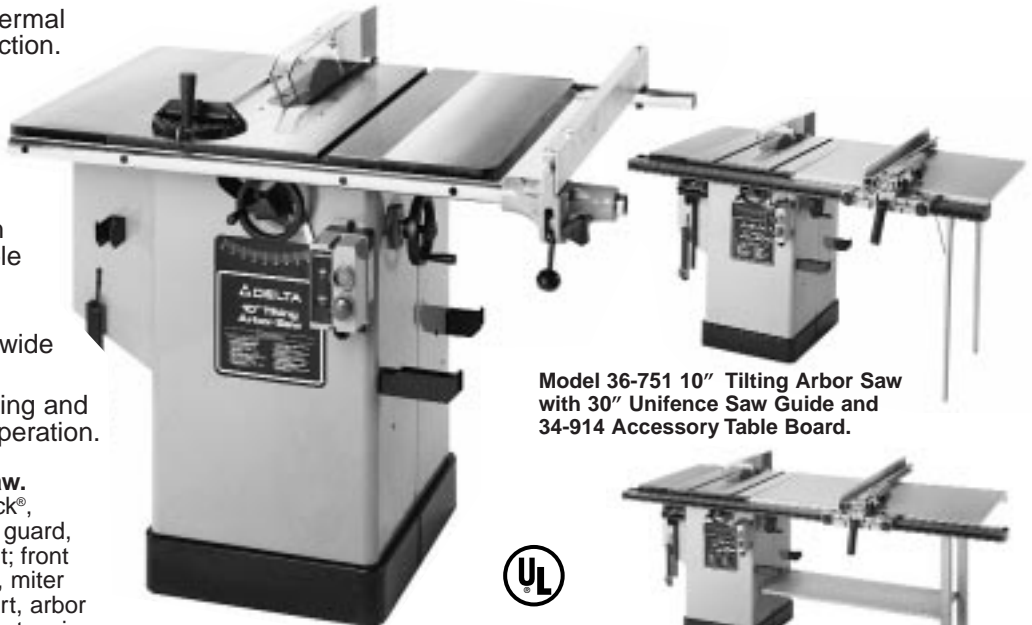
Model 36-755 10" Tilting Arbor Saw
