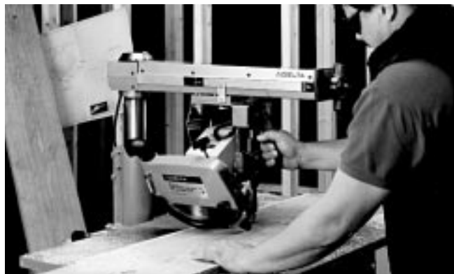
Positive bevel and miter stops at commonly used angle positions.
