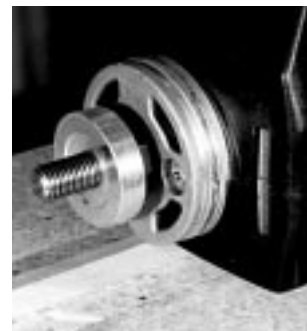
Features a dual shaft (threaded 5/8"-12LH and 1/2"-20RH) for maximum utilization of accessories.
