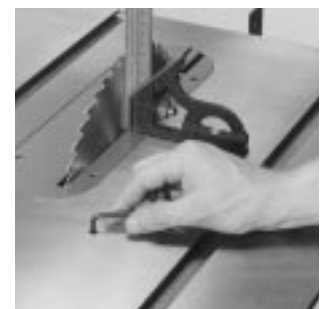
Unique "table top located" adjusting screws for accurate setting of 45° and 90° positive blade stops.
