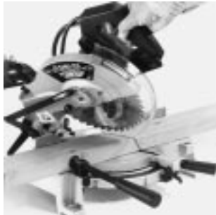
Versatile tilting blade allows you to bevel cut a nominal 2 x 6 at 45°, compound angle cut a 2x4 at 45° miter and 45° bevel cutting position.
